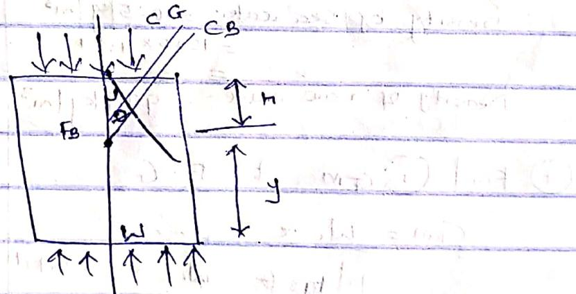
Example :- A ship of total mass 5000000 kg floating on the sea in a stable condition a portion of the cargo of mass 25000 kg ship through a distance of 6m off at
